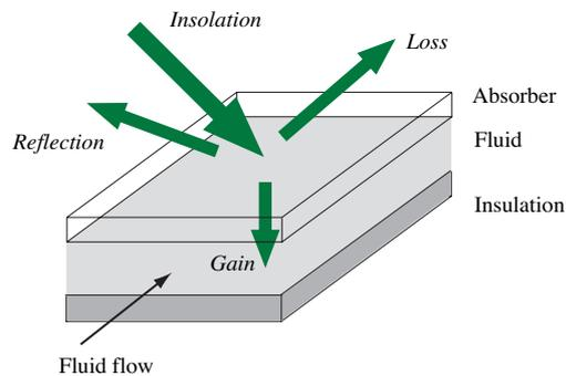
Basically, a thermal solar collector of the type discussed here is a flow heater (see Chapter 8 for a treatment of uniform models of flow heaters). Unlike the models introduced in Chapter 8, the ones created here will take into account the spatial variation of temperature of the fluid in the duct.
