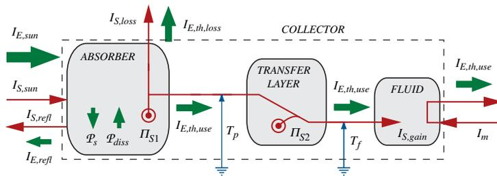
**Figure 14.3:** Process diagram for the collector showing fluxes of entropy and energy. Almost all the entropy transferred to the fluid and to the environment is produced in the system.
