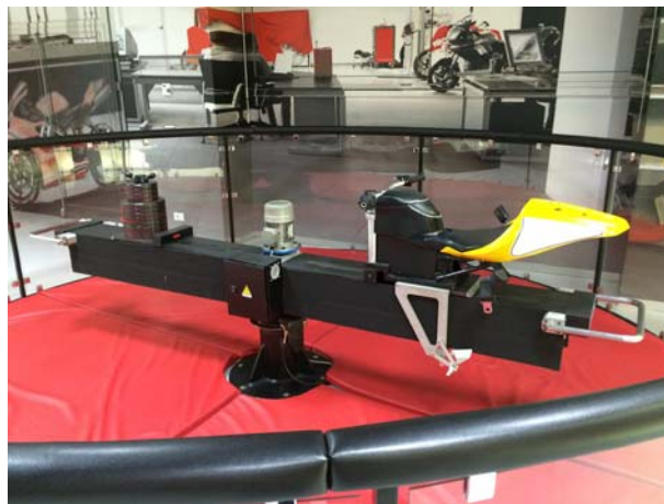
Fig. 1: The Carousel of Angular Momentum workstation. Note the beam, seat, counterweights, and the vertical axis of rotation.
