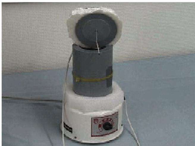
Figure 8: Experimental setup for the final project of Part IV: Cooling of hot water in a thick-walled PVC container. There are two thermometers, one for in the container, the other mounted on the outside wall of the PVC tank.
