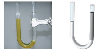
Figure 1.2: With oil on top of water in the right column of the U-pipe, the levels of the liquids are not the same after equilibration. The effect is observed as well if the two tanks have different cross sections and/or different shapes.
