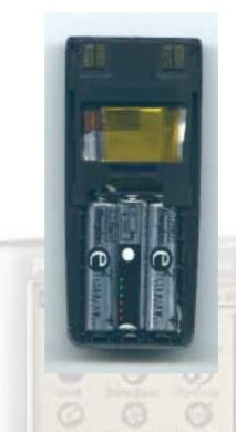
Telcordia's patented Flat Supercapacitor
