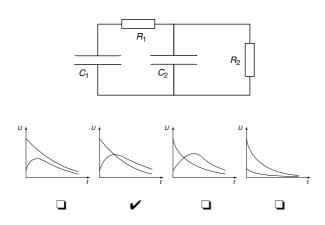
Explanation: U1 must become larger than U2 at one point for discharging to continue. The maximum of U1 must occur when U1 = U2.
