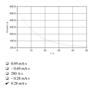
Explanation: Transported charge from area between curve and t-axis:  $Q_e \approx 2.75 \cdot 10^{-4} \text{ A} \cdot \text{s}$
