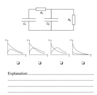
2. Two capacitors and a resistor are connected in a circuit as in the figure. The capacitance of the first capacitor is 100  $\mu$ F, that of the second is 200  $\mu$ F. At the beginning the voltage across each of the capacitors is 5.0 V. The resistance is 20 k $\Omega$ .
