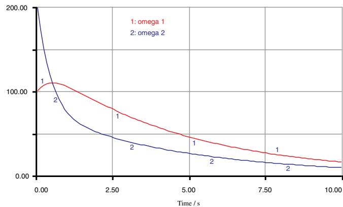
The mechanical system is analogous to two communicating straight-walled fluid containers, where the second container has an outflow. The second container has a smaller cross section, and it is filled to a higher level initially. The parameters of the system give the time constant a value of around one second.
