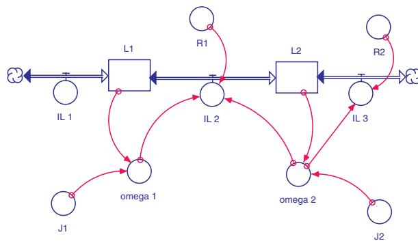
The diagram represents the two laws of balance of angular momentum (the wheels store angular momentum). The angular velocities are calculated from the values of angular momentum, and the momentum currents (2 and 3) are proportional to angular velocity differences.
