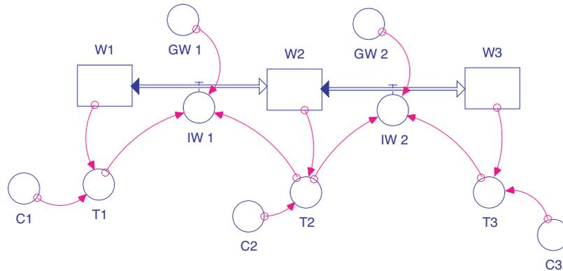
d. Neglect the effect of the thin metal wall separating two bodies of water, only take into account the convective transition layers on either side:  $G_W = A \cdot h = 0.10 \cdot 0.10 \cdot 1 / (1/400 + 1/400)$  W/K = 2.0 W/K.
