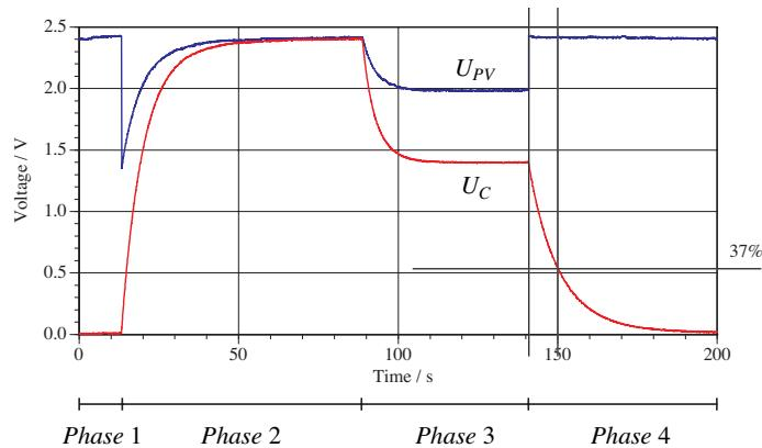
h. The capacitance of the capacitor can be determined with the help of the time constant of the right loop:
