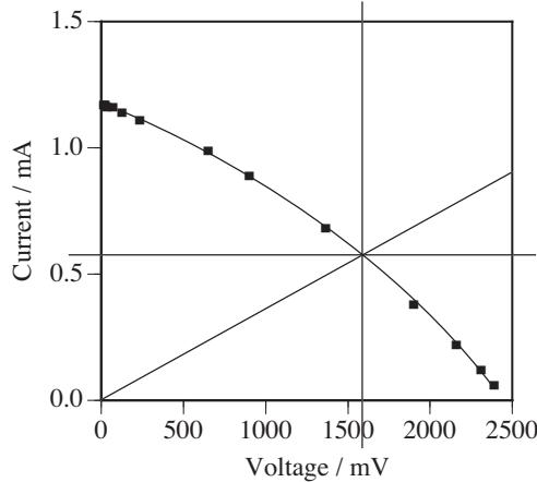
e. A change in the capacitance of the capacitor does not lead to a change of the voltage of the PV panel at this point. This is so since the capacitor is uncharged at the beginning, i.e., its voltage will be zero at the beginning irrespective of the capacitance. Put differently, voltages and current are determined only by the PV panel and by the resistor.
