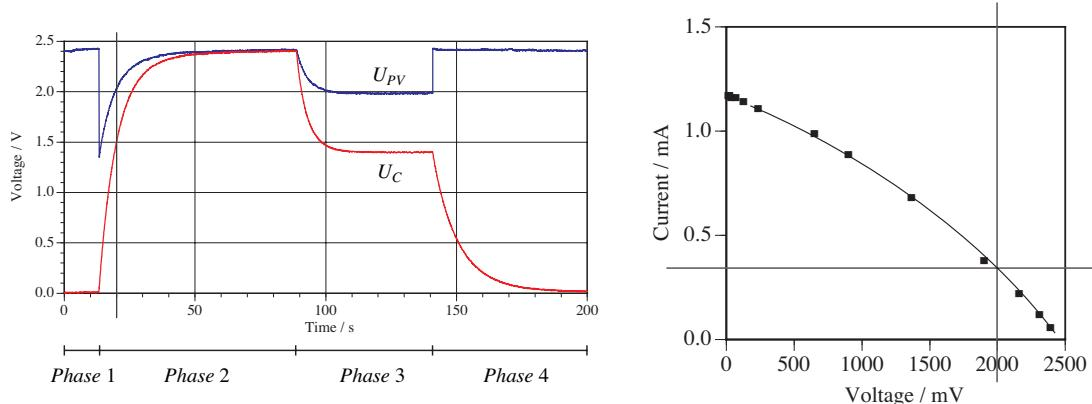
From graph:  $U_C(t = 20\text{s}) = 1.5 \text{ V}$ . Current of energy going into the capacitor:  $I_{W\_C} = U_C \cdot I_{Q\_PV} = 1.5 \text{ V} \cdot 0.33 \text{ mA} = 0.50 \text{ mW}$ . Therefore, energy is dissipated in the resistor at a rate of  $0.67 \text{ mW} - 0.50 \text{ mW} = 0.17 \text{ mW}$ .
