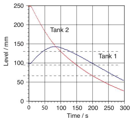
c. If  $h_1 = H_1$ , then  $\Delta p_{C1} = 0$ , therefore  $I_{V1} = 0$ , therefore  $dV_1/dt = 0$ , therefore  $H_1$  has its maximum there.
