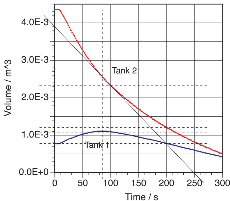
$$\begin{aligned}\frac{d}{dt}V_2 &= I_{V1} - I_{V2} \quad , \quad I_{V1} = 0 \\ \frac{d}{dt}V_2 &= -I_{V2} \\ \frac{d}{dt}V_2 &\approx \frac{-3.9 \cdot 10^{-3}}{250} \frac{\text{m}^3}{\text{s}} = -1.6 \cdot 10^{-5} \frac{\text{m}^3}{\text{s}} \quad \Rightarrow \quad I_{V2} = 1.6 \cdot 10^{-5} \frac{\text{m}^3}{\text{s}}\end{aligned}$$
